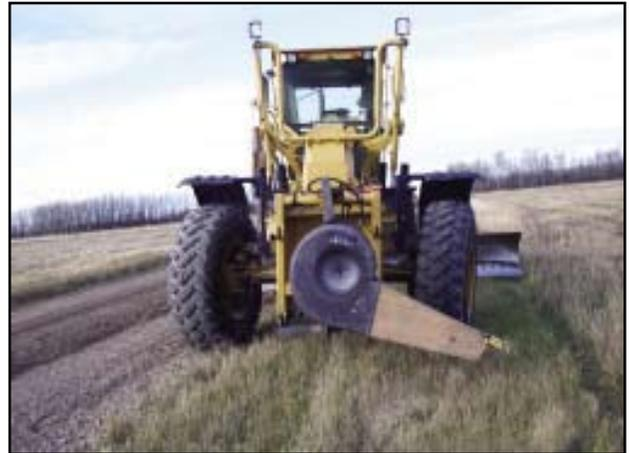
**Solution** A blower attachment on the front end of a motor grader can blow the grass clippings off the gravel surface and out of the way of the moldboard, preventing clippings from mixing with the gravel.
