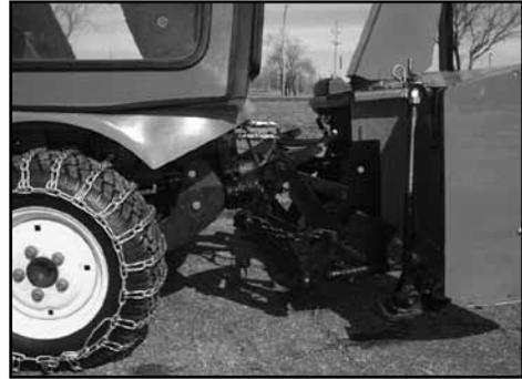
**Problem** Operators using tractor-mounted snow blowers to clear city sidewalks often had to make a second pass over the blowing area to clear remaining snow. Driving over cracks in the sidewalk or slight changes in elevation jolted the operator, posing safety concerns, and also left snow behind on the plowed surface. A lack of traction was also an issue for operators, even with chains installed on the equipment.
