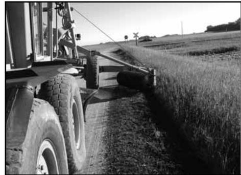
**Problem** The gravel from gravel roads or shoulders is often pushed out and down the slopes of Sibley County roads, causing rough conditions and pavement edge drop-offs. For gravel shoulders on paved bituminous highways, two motor graders were used in reclaiming operations, one with a retriever and the other to blade the gravel back onto the shoulder. This process was expensive in terms of budget and personnel, as it required two graders and operators.
