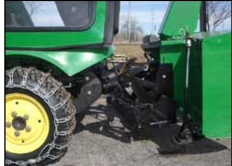
**Problem** Operators using tractor-mounted snow blowers to clear city sidewalks often had to make a second pass over the blowing area to clear remaining snow. Driving over cracks in the sidewalk or slight changes in elevation jolted the operator, posing safety concerns, and also left snow behind on the plowed surface. A lack of traction was also an issue for operators, even with chains installed on the equipment.
