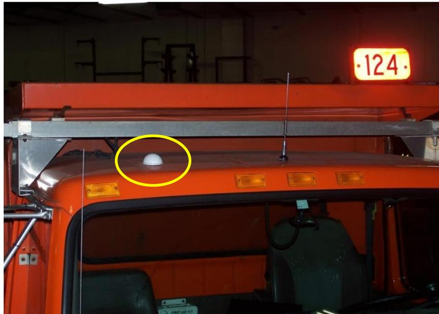
**Figure 6: GPS preemption unit and control panel**
