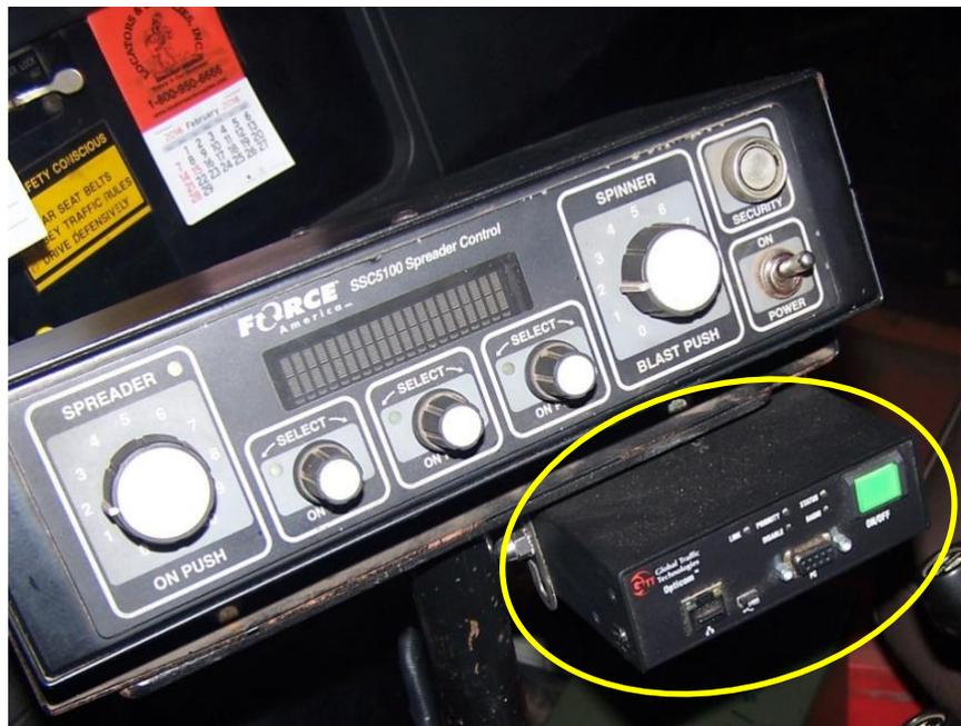
The second piece of equipment is the GPS preemption unit and control panel that allows the operator to turn the GPS preemption system off and on. A small cable runs between the antenna and the control panel. See figure 6.
