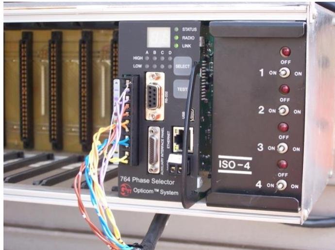
**Figure 2: GPS Phase selector card installed in cabinet**
