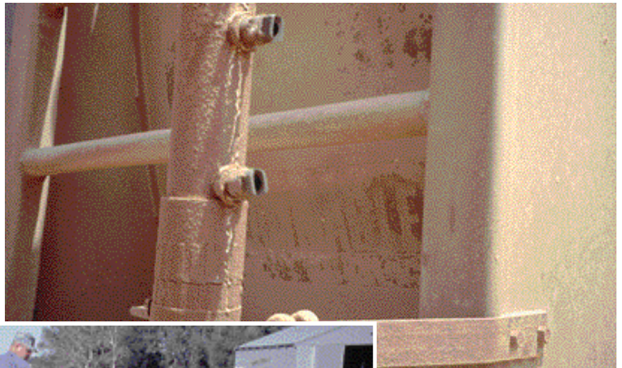
This photo shows part of the spray bar with spraying nozzles.
