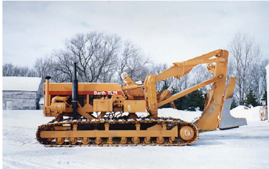
Example of a machine called a tile plow that is commonly used in some regions to install polyethylene pipe into farm fields for drainage purposes. This type of machine has also been used to plow drain tile into gravel roads with great success in some areas.
