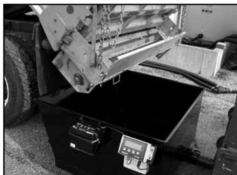
**Problem** During the winter months, Olmsted County uses 17 tandem-axle snowplow trucks to maintain 530 miles of roadway. The county was unable to verify the amount of salt and sand being applied to the roadway by these vehicles because it lacked a uniform method for calibrating the sanders on each truck. It was difficult to determine if the amount of salt and sand applied was sufficient or if the county was overspreading the material.
