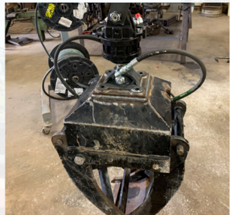
The Otter Claw has an omnidirectional hydraulic swivel head.
